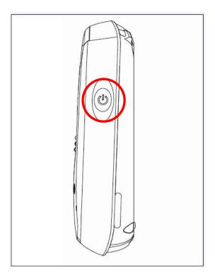
Turn On MD4 by pushing and holding the power button until the device vibrates.
