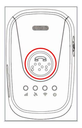
In order to initiate an emergency or SOS notification, press and hold the SOS button for 3 seconds or until you feel the MD4 vibrate (this is a default setting that can be customized). At that point the MD4 will do the following:
