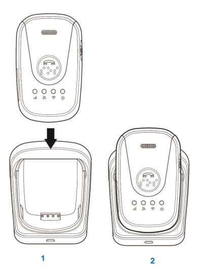
Before First Use: Ensure a fully charged MD4 upon receipt by docking it in the charging cradle prior to use. It may take 3 hours to ensure a full charge. The power icon will light-up in orange when charging and the power icon will flash when fully charged. After fully charging the MD4, based on standard settings and usage it should last 2 full days before requiring another charge.
